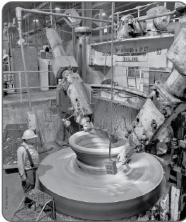
1965 built, Dual Tool 4000 mm VTL at Frog Switch Foundry, Carlisle, Pennsylvania, USA
