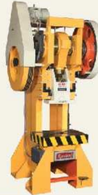
Mechanical Power Press
