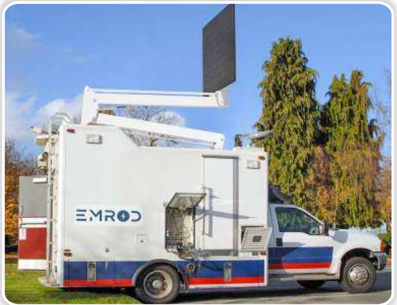
Conceptual photo-illustration of an antenna truck outfitted to supply wireless power to disaster areas
